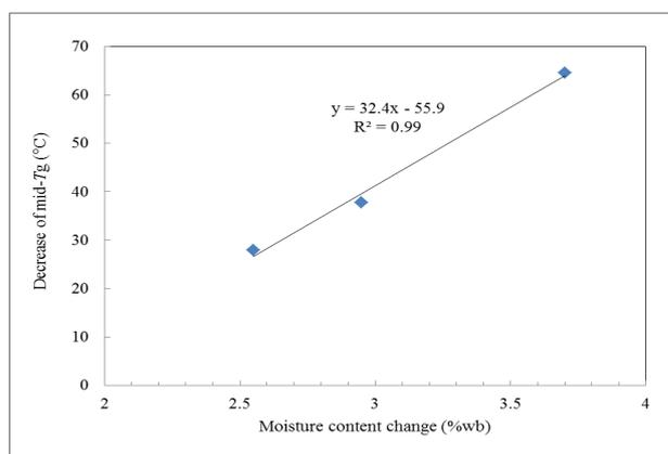
Figure 1. The plasticization effect of water in suppressing the  $T_g$  of amorphous saccharide mixture systems
