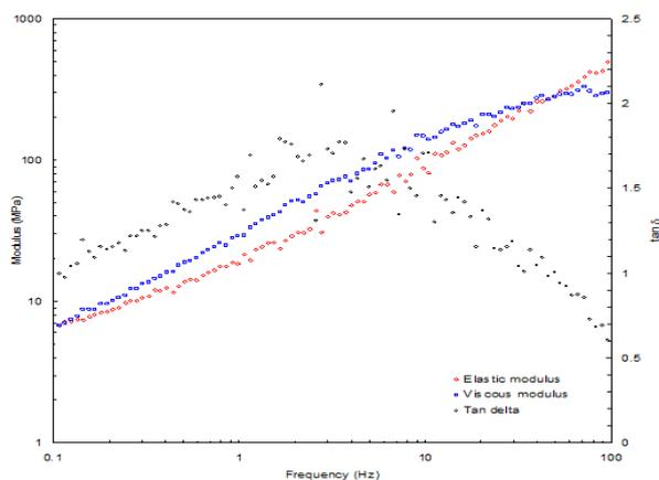
Figure 2. Representative dynamic moduli and  $\tan \delta$  as a function of frequency for the rubbery saccharide mixture with SC/MD of 7/3. Data were obtained at 25°C.
