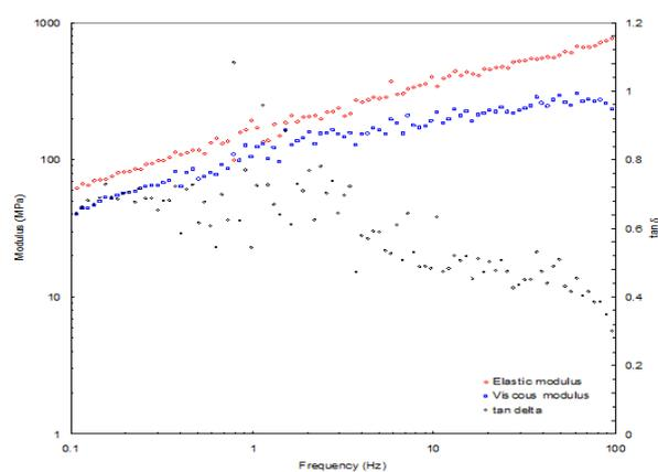
Figure 3. Representative dynamic moduli and  $\tan \delta$  as a function of frequency for the rubbery saccharide mixture with SC/MD of 3/7. Data were obtained at 25°C.
