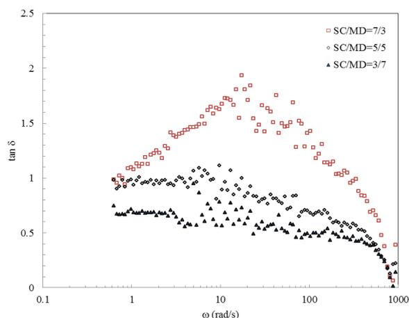
Figure 4. Frequency dependence of  $\tan \delta$  for rubbery saccharide systems. Data are means of two replicates obtained at 25°C.
